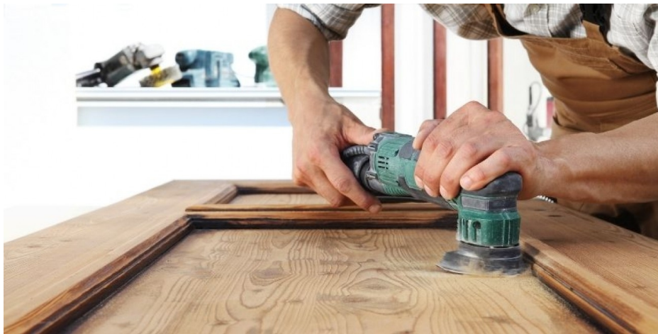
Fig. 2.36: Sanding and Surface Preparation
