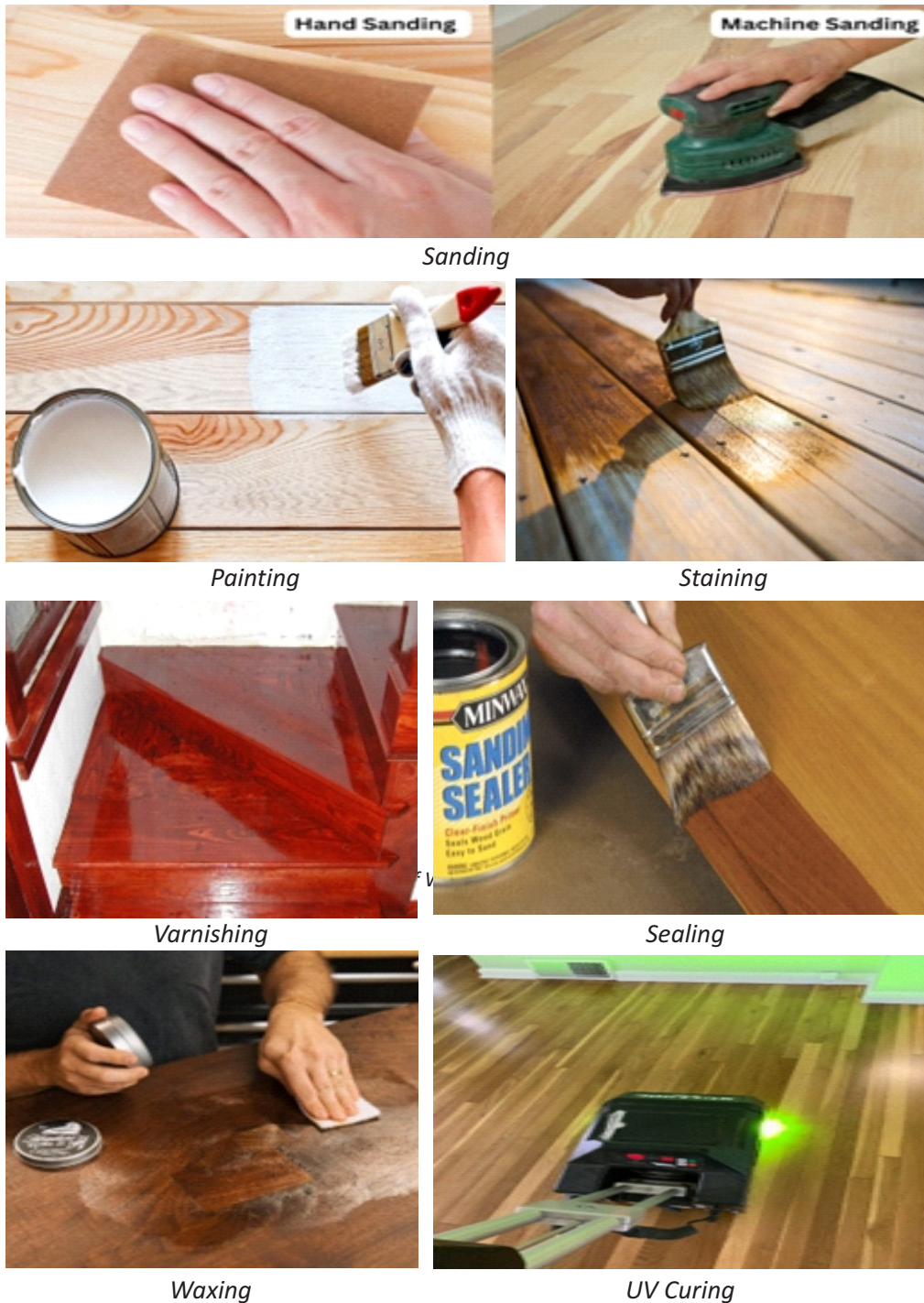
Fig. 2.40: Different Wood Finishing Techniques
